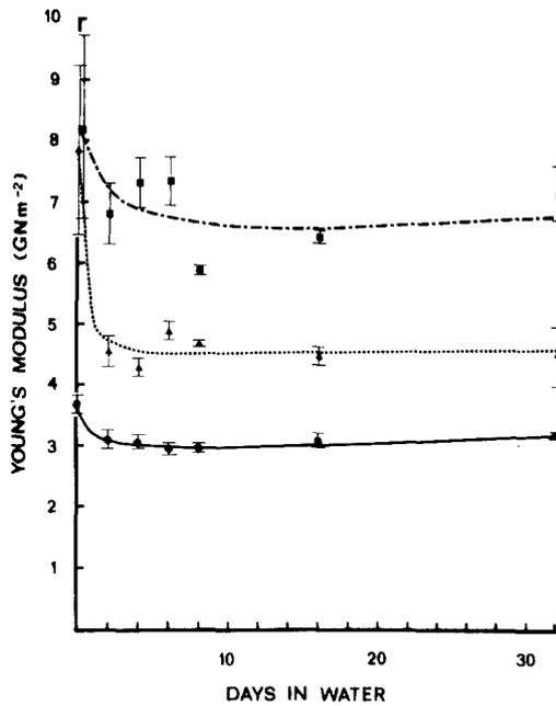
Figure 7 Moduli of bis-GMA/TEDMA and 40 vol% glass bead composites as a function of immersion time in water.
