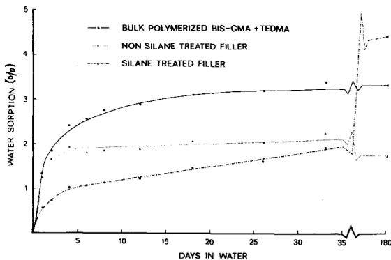
Figure 8 Water uptake by weight gain against immersion time at  $60^\circ\text{C}$  of bis-GMA/TEDMA and 40 vol% composites.
