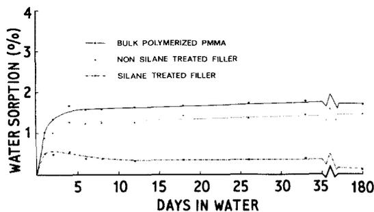
Figure 4 Water uptake by weight gain against immersion time at 60°C for PMMA and composites.
