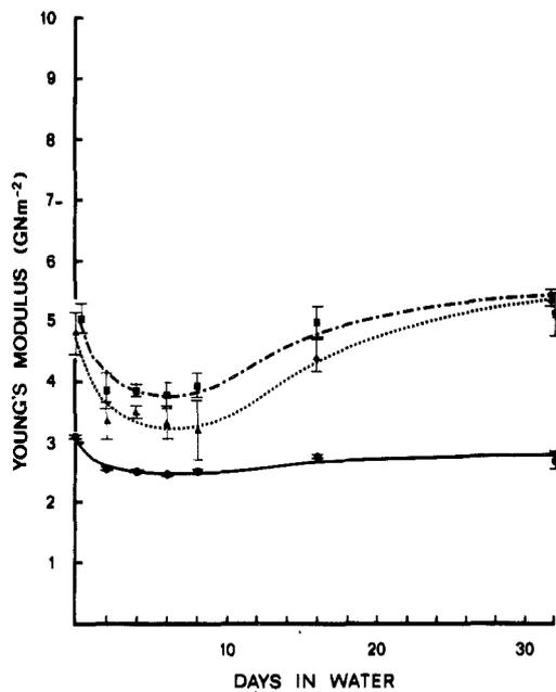
Figure 3 Moduli of PMMA and 40 vol% filled PMMA composites as a function of treatment time in water.
