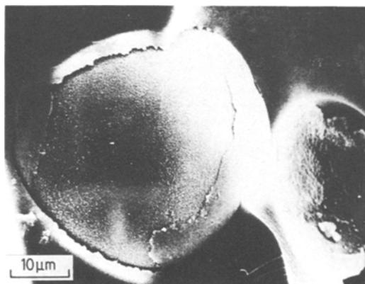
Figure 11 Bis-GMA/TEDMA containing 40 vol% untreated glass beads. Fractured after 180 days in water at 60°C.
