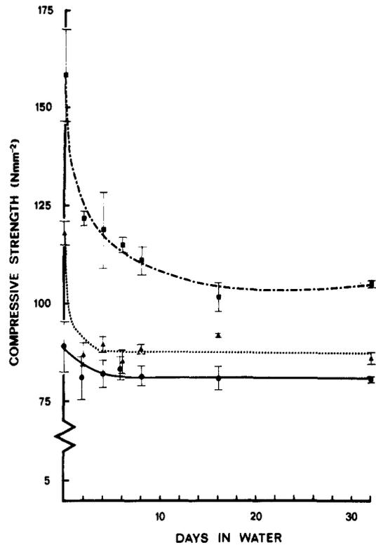
Figure 9 Effect of  $60^\circ\text{C}$  water immersion on compressive yield strength of bis-GMA/TEDMA and composites.
