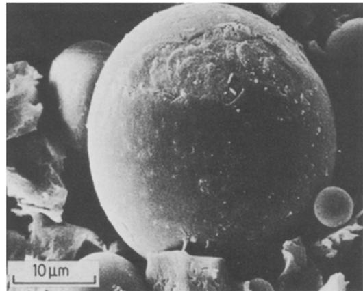
Figure 10 PMMA containing 40 vol% untreated glass beads. Fractured after 32 days in water at  $60^\circ\text{C}$ .
