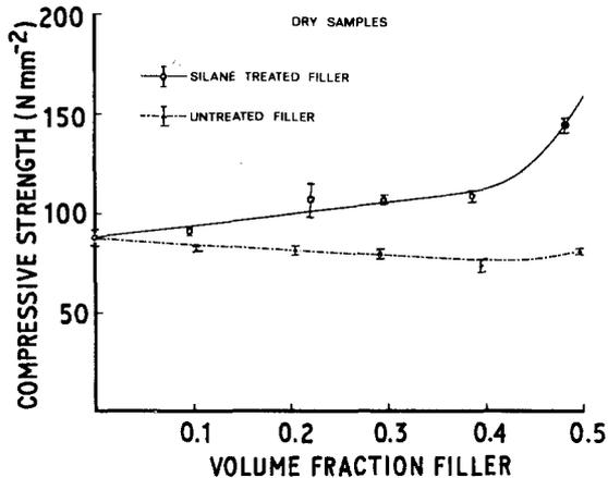
Figure 5 Compressive yield strength (0.2%) against filler volume fraction for dry PMMA composites.
