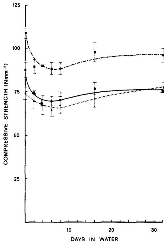
Figure 6 Effect of 60°C water immersion on compressive yield strength of PMMA and composites.
