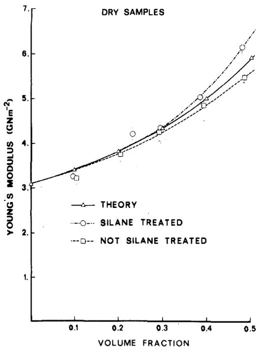
Figure 1 Modulus in compression against volume fraction of glass bead filler (silanated or untreated) in PMMA. Theory according to Equation 1, series model.
