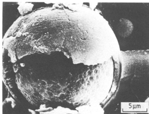
Figure 12 PMMA containing 40 vol% untreated glass beads. Fractured after 180 days in water at 60°C.
